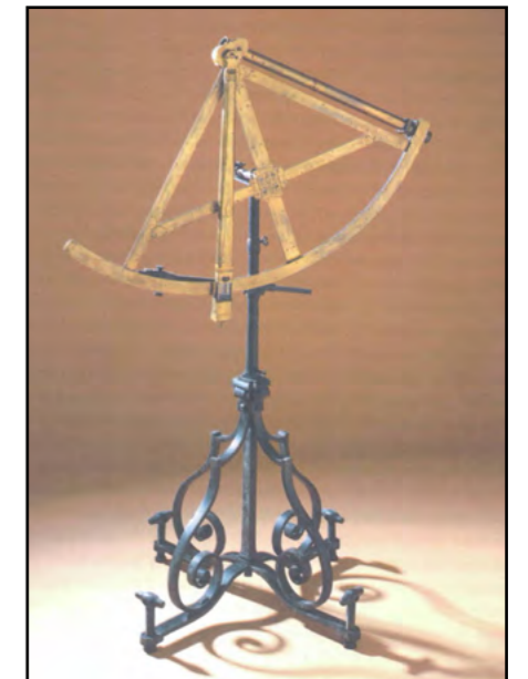
Fig. 1. Quadrant by Butterfield, radius 58cm, similar to the one given to the emperor by the King's mathematicians
