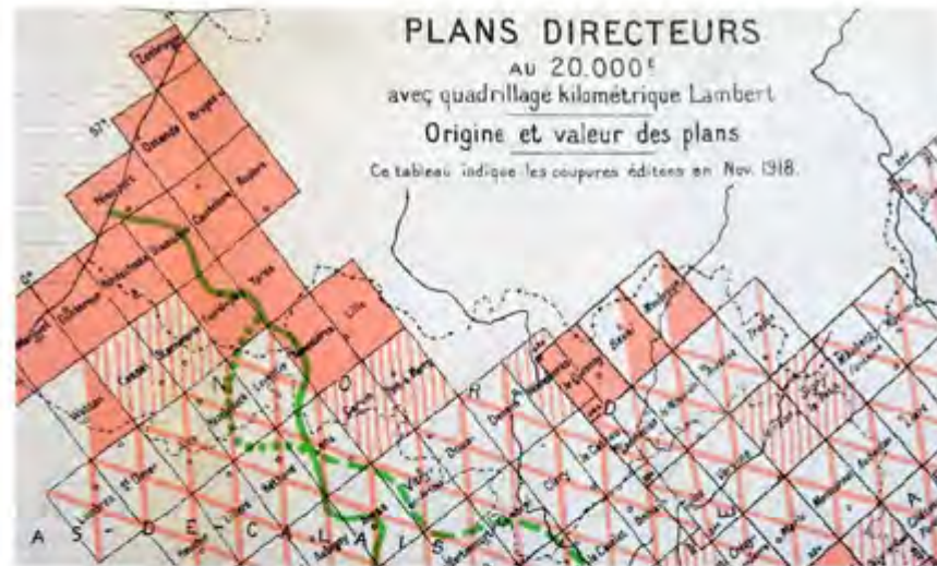
Fig. 4. Origin of the French 'Plans Directeurs' produced during WW I: pink plans are totally based on large scale surveys, hashed ones only partially; crossed ones are based on cadastral surveys, aerial photographs, etc.
